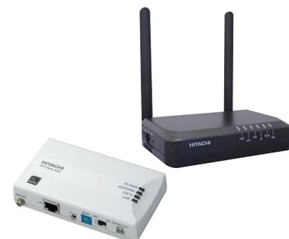
CPTrans series of LTE-enabled IoT/M2M terminals
